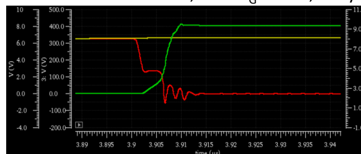
Discrete FET and drive, with R G = slow, lossy
