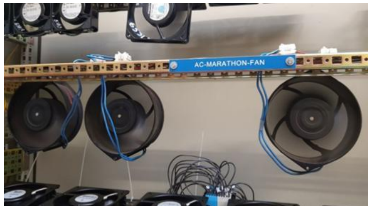
Marathon test for endurance runners, some of which have been in operation since the 1980s.
