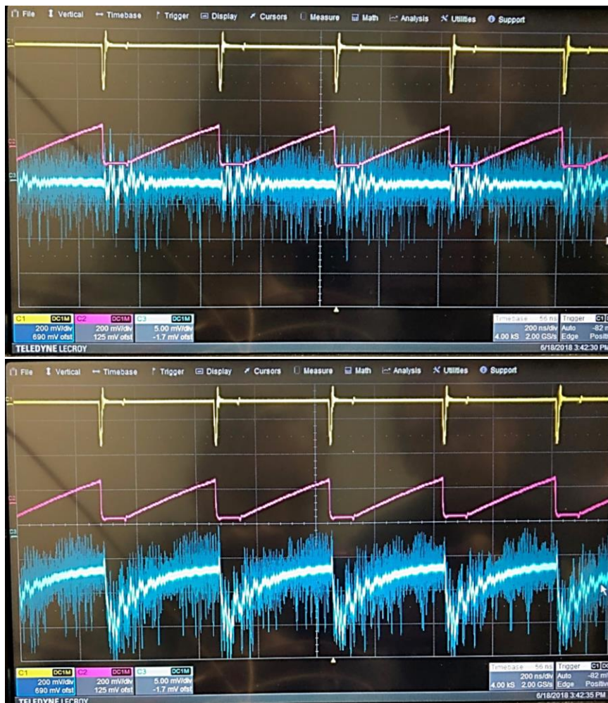
Figure 8: The top panel of the oscilloscope shows the cross talk which may be observed on the APD (blue). The bottom panel shows the APD with the laser focused on the detector region (blue).
