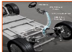
Steer By Wire, SBW and Electric Power Steering, EPS (AS5147, AS5247 - dual die version)
