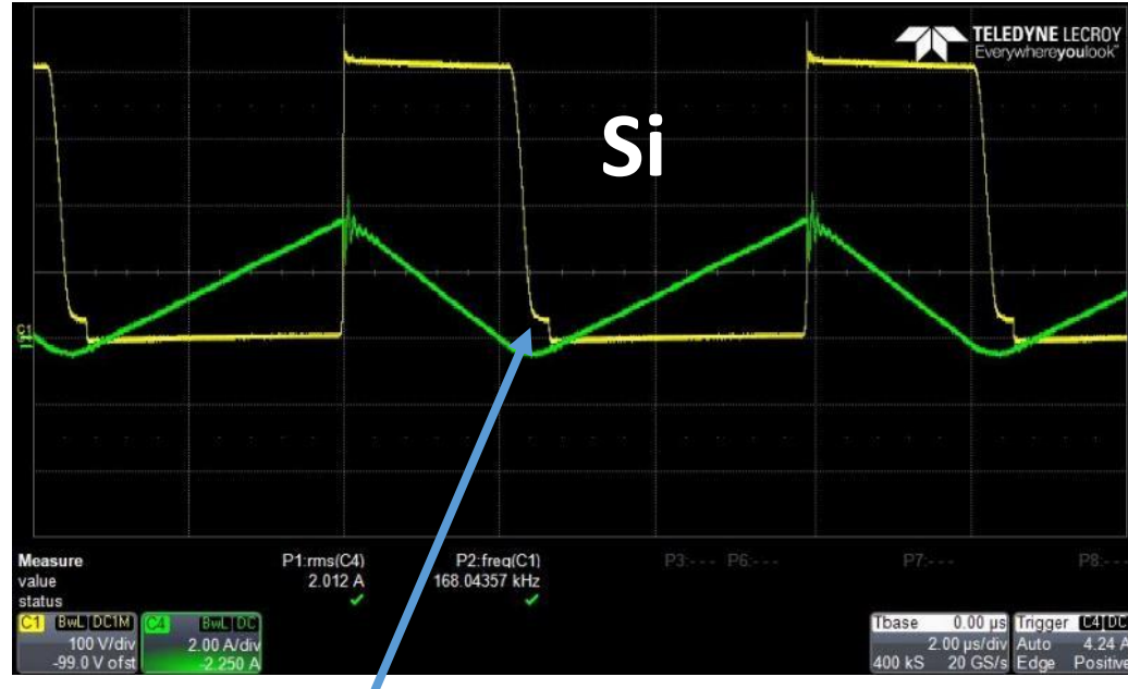
120V AC , Si CP partial hard-switching (~200kHz)
